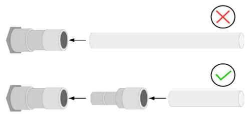
Directly plugging and pulling a telfon hose more than once may lead to particle contamination which can affect the measurement. For this please use the included adapter plugs and keep them on your tubes.
