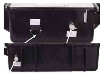
1. Unscrew the protection caps at inlet and outlet.
