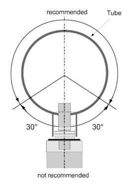
Please install the sensor only in the recommended area like you can see in the picture. An upside down installation is not permitted. Please consider that the distance to the vertical level must be  $>30^{\circ}$ .
