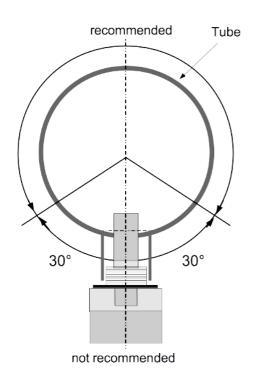
Please install the transmitter only in the recommended area as you can see in the picture. An upside down installation is not permitted. Please consider that the distance to the vertical level must be >30°.
