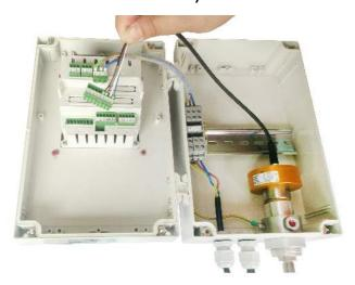
1. Open the S305 case and remove the sensor cable connected at the display terminal first. See the left picture.
