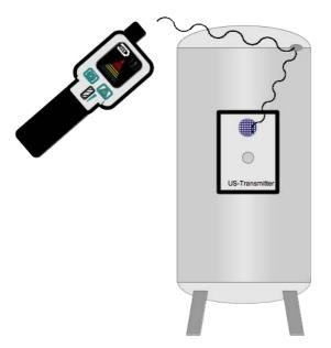
For example Leak test at a tank:
