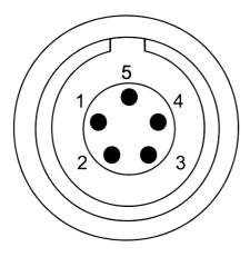
Connection pins (view onto the connector)
