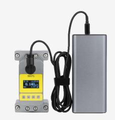
S462 powered by external power bank with connection cable A553 0156
