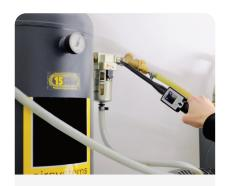
Scan with the focus tube and focus tip the roughly location till the exact location is found.
