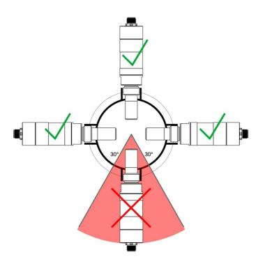
Install the device only in the recommended area, as shown in picture on the left.
