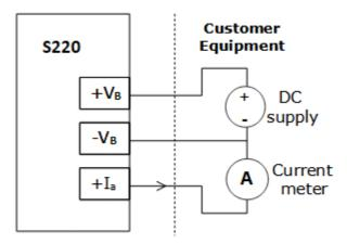
3-wire analog and Modbus/RTU outputs
