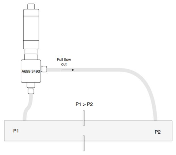
**Remark:** Ensure that the teflon hose remains dry and clean. Wet and contaminated hoses can effect the measurement and should be exchanged.
