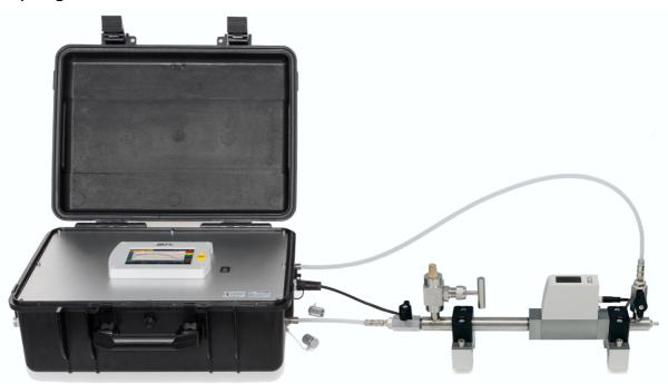
Please connect the isokinetic sampling device using the teflon hose delivered with the device. The following illustrates which outlets of the sampling device need to be connected to which inlets of the S600.
