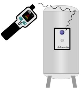
For example Leak test at a tank:
