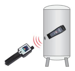
For example leak test at a tank:
