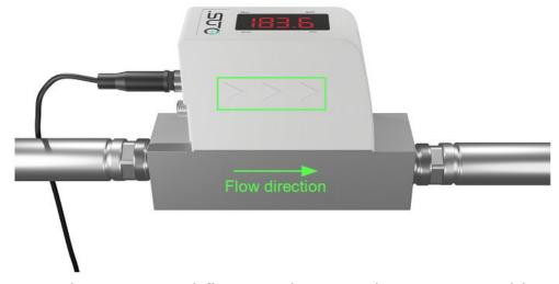
Due to the integrated flow conditioner, there are no additional straight pipe requirements for good measurement. However for best measurement, it is recommended 3-5 times inner diameter straight pipe at the inlet.
