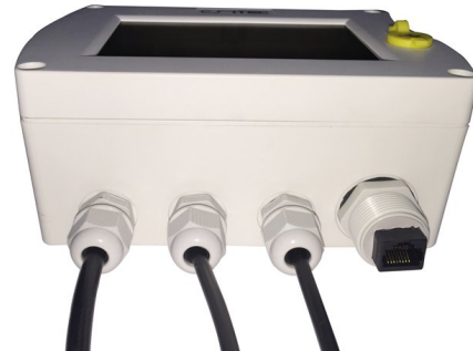
External RJ45 connector (IP65)
